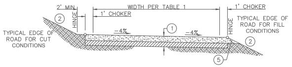
OPTION 2: GRAVEL ROAD SECTION WITH CONSTANT CROSS SLOPE
